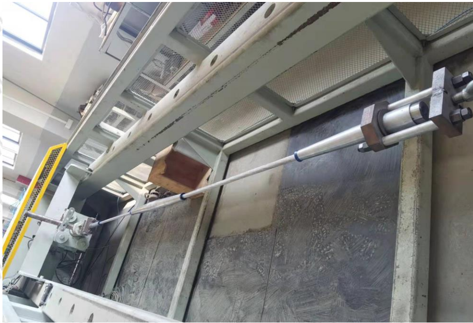
Maximum Load test of #636 MCM ACSR conductor test site photo
